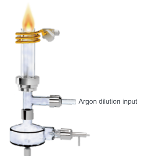
Schematic diagram for argon dilution input
